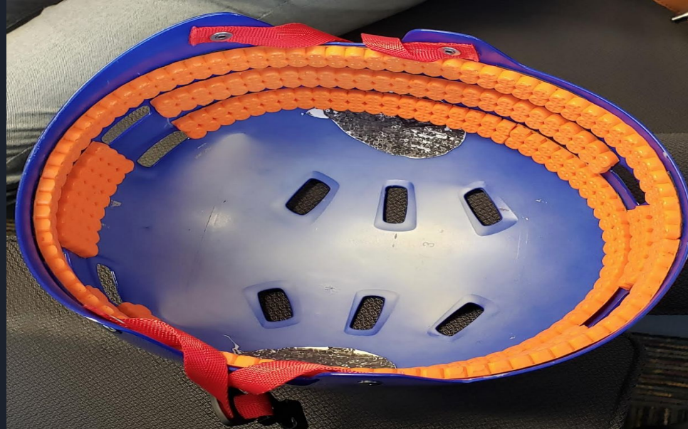
Figure 7: Helmet Shell With D30 Material
